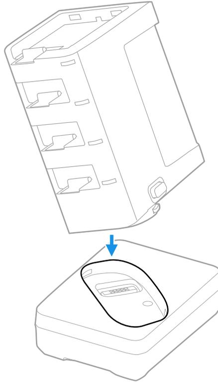
2. Press the latch release button as you push the battery charger down until it snaps in.
