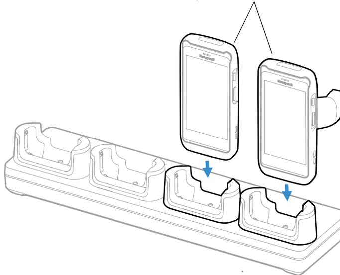
**Note:** Bases CT40-CB-PB and CT40-NB-PB will not charge unless a boot is attached to the computer.
