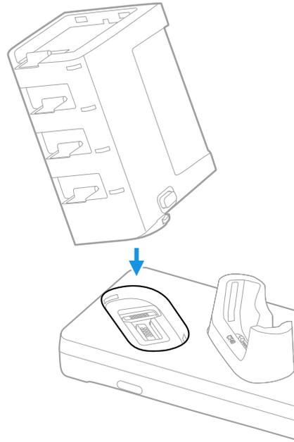
2. Press the latch release button as you push the battery charger down until it snaps in.
