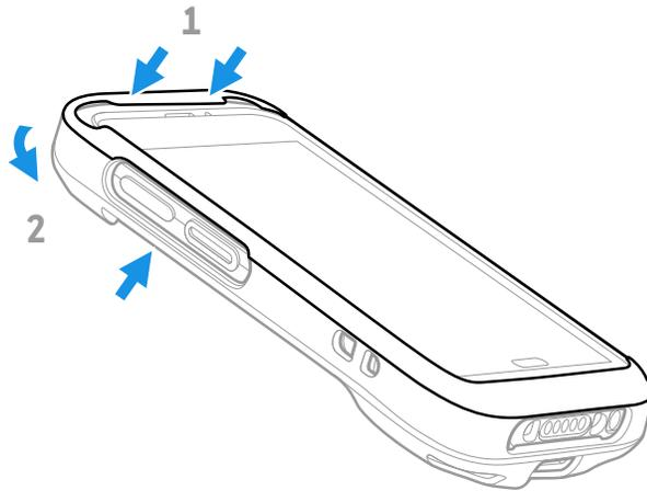
3. Lift the unit up and out of the bottom of the boot.
