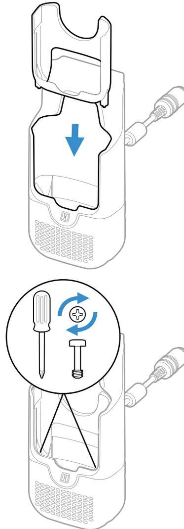
2. Insert the computer with a wireless battery installed into the wireless vehicle dock.
