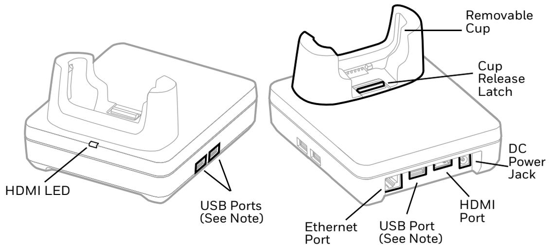
**Note:** The display dock supports USB direct connections only. The dock does not support USB hub connections, including keyboards with USB port(s).
