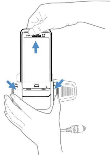
**Note:** After removing a computer from a CT45-VD-CNV-SPK vehicle dock, wait at least 5 seconds before reinserting it. This pause will allow time for audio to transfer from the computer speaker back to the dock speaker.
