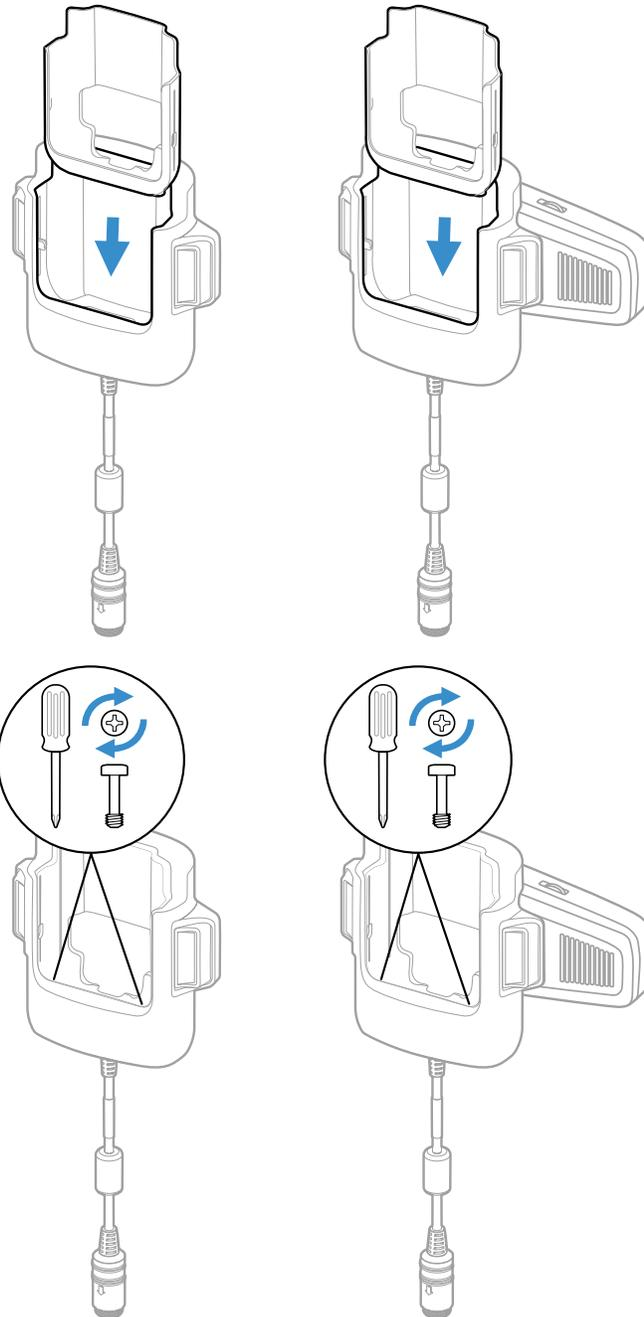
2. Pushing down firmly, insert the computer with a battery installed into the vehicle dock.
